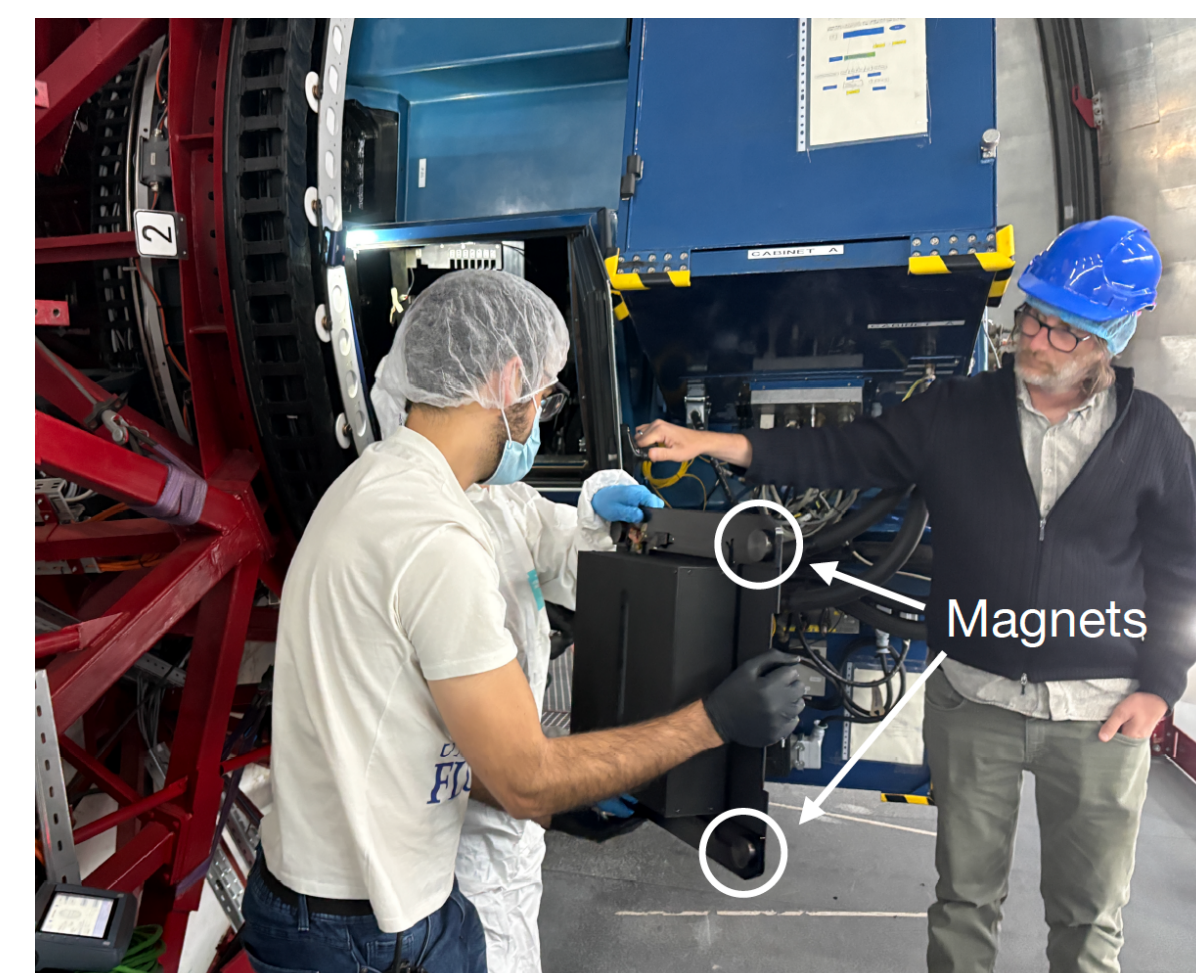
Left: Manual insertion of MAAT into the OSIRIS+ mask-loader, showing the magnetic interface. Right: MAAT installed in the OSIRIS+ mask-loader, positioned next to the standard OSIRIS+ long-slit masks.
